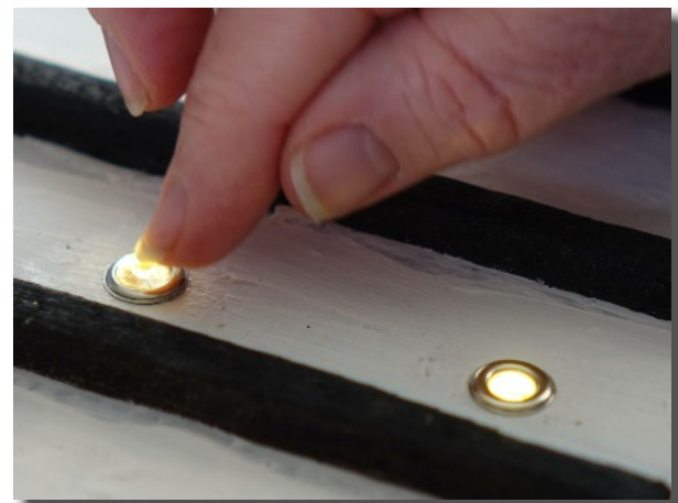
I made the downlighters from 5.5mm poppa eyelets and glass beads and a string of led lights, all fitted nicely together
